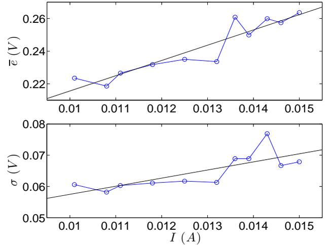
Fig. 5: The mean value  $\bar{e}$  (up) and the standard deviation  $\sigma$  (down) at fixed current  $I$  is plotted against  $I$ . A linear fitting is performed over the range available.
