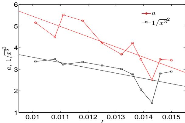
Fig. 6: The asymmetry coefficient  $a$  is obtained for each  $I$  by fitting the histogram with a GG distribution.  $a$  is plotted against the current  $I$ , together with the inverse squared skewness.
