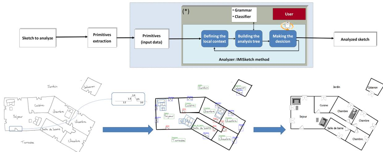
Figure 1. Synthetic scheme of IMISketch method for structured documents interpretation
