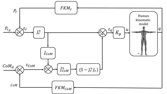
Fig. 4. Block diagram of the proposed control scheme.
