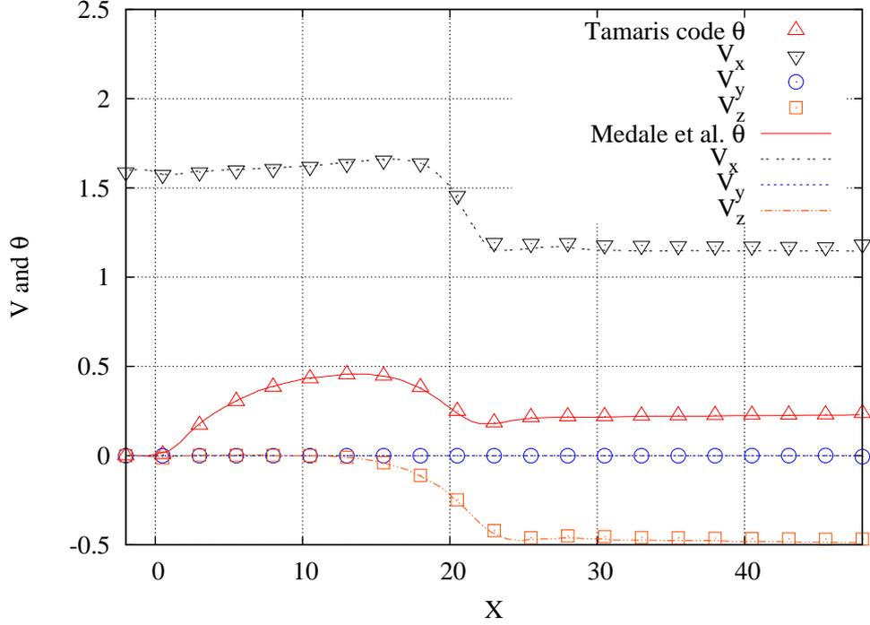
Fig. 3: *The longitudinal profiles of the rescaled variables  $V_X$ ,  $V_Y$ ,  $V_Z$  and  $\theta$  (represented by symbols) along the axis ( $Y = 5$ ,  $Z = 0.5$ ) compared with the reference solution (Nicolas et al., 2011) (lines).*
