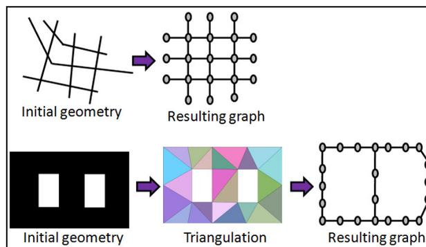
**Fig. 7.** Example of graph computation
