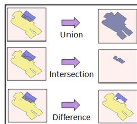
**Fig. 4.** Example of union, intersection and difference actions.
