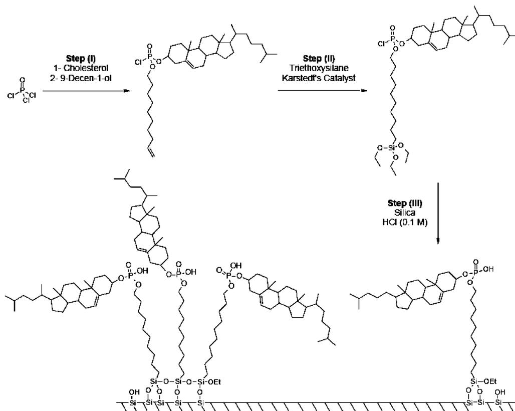
Fig. 1 Synthetic pathway of the PCP
