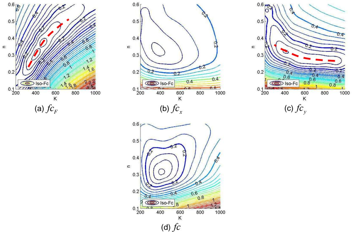
Figure 3 : sensitivity analysis of hardening parameters by kriging response surfaces, evolution of the four objective functions based on: (a) load-displacement, (b) displacement field  $U_x$  in the tensile direction, (c) displacement field  $U_y$  in the transverse direction, (d) total objective function
