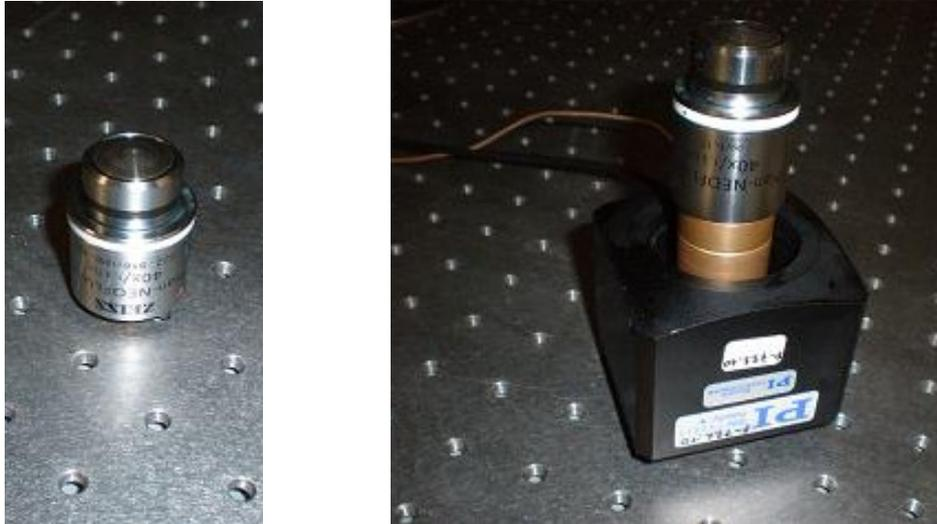
**Figure 28** *1.3 NA oil objective (ZEISS) mounted on an extension screwed on piezoelectric stage.*
