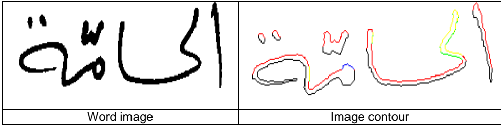
Figure 10: Contour feature extraction
