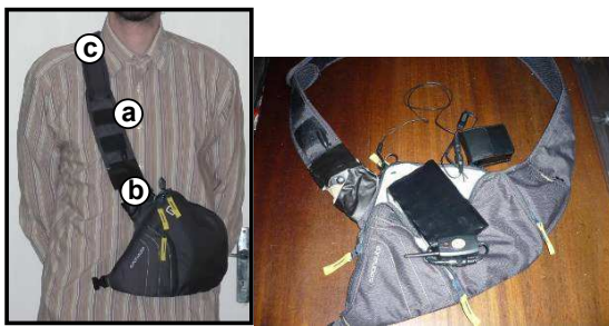
Fig 3. Illustration of the current prototype, with considered camera position (a,b,c). The system is composed of a strap bag which holds a battery, a camera, a microphone, and a wireless transmitter.
