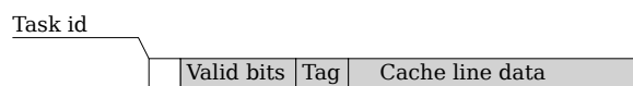
Figure 2: Storage requirements for PRETI caches: each cache line is extended with a task id .
