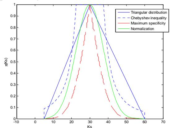
Figure 4. Comparison of the four different possibility distributions used for  $K_s$ : triangular function (Section 4.1), Chebyshev inequality (Section 4.2), principle of maximum specificity (Section 4.3.1), normalization of the probability density (Section 4.3.2).
