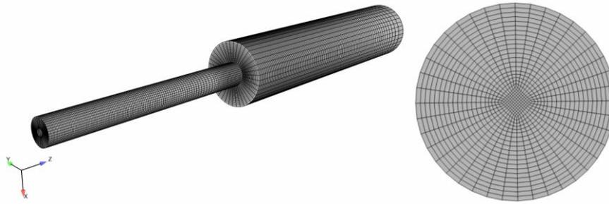
Figure 2. Computational grid of the plasma torch.
