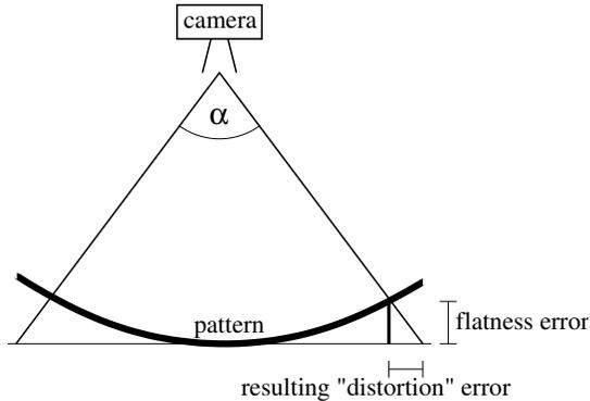
**Fig. 7:** A flatness error in the pattern can be mistaken for a “distortion”. In the experiments, with  $\alpha \approx 65^\circ$  and a flatness error about  $100 \mu\text{m}$ , the produced “distortion” error is about  $64 \mu\text{m}$  (flatness error  $\times \tan \frac{\alpha}{2}$ ). Our pattern has the size  $406 \times 271 \text{ mm}$  and produces a  $1761 \times 1174$  image, then one pixel corresponds to  $230 \mu\text{m}$ . Thus the observed error would be approximately 0.3 pixel.
