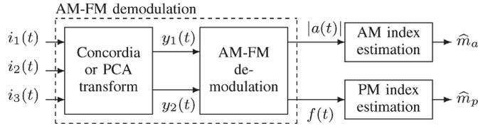
Fig. 1. Block diagram of the proposed technique. Symbols  $i_k(t)$  ( $k = 1, 2, 3$ ) correspond to the stator currents,  $|a(t)|$  and  $f(t)$  correspond to the instantaneous amplitude and frequency, and  $\hat{m}$  corresponds to the modulation-index estimate.
