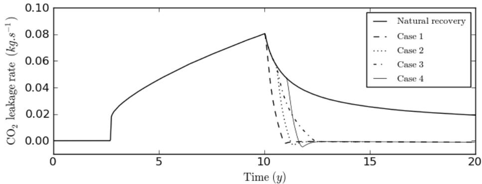
Figure 3: CO<sub>2</sub> leakage rate. The CO<sub>2</sub> injection stops at 10 years and various cases of hydraulic barriers are experienced. Cf. Table 2 for the description of the cases and results.
