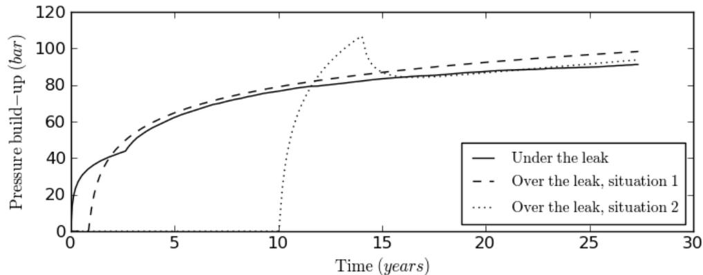
Figure 5: simulated over-pressure under the leak created by the CO<sub>2</sub> injection and analytical pressure build-ups above the leak created by the designed hydraulic barriers. Situation 1: a 30 m<sup>3</sup>/h brine injection starts at 300 days. Situation 2: brine is injected at 50 m<sup>3</sup>/h from 10 to 14 years, and at 30 m<sup>3</sup>/h after.
