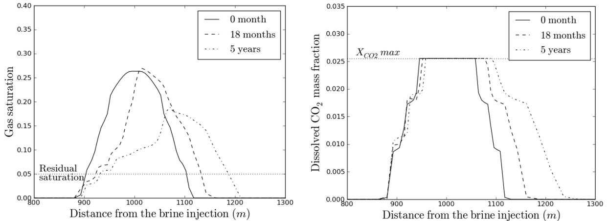
Figure 4: Gas saturation (left) and CO<sub>2, aq</sub> mass fraction (right) in the upper aquifer (average of the three layers) in a vertical cross-section from the brine injection well (located at 0m) to the leak (locate at 1000 m) after 0, 1.5 and 5 years of brine injection at 15 m<sup>3</sup>/h
