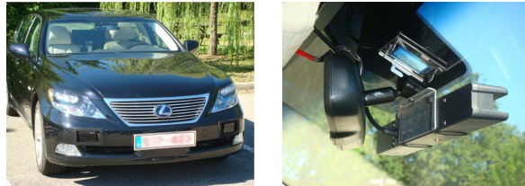
Figure 4: The experimental vehicle is a Lexus LS600h, equipped with a TYZX stereo camera, and two IBEO Lux laser scanners.
