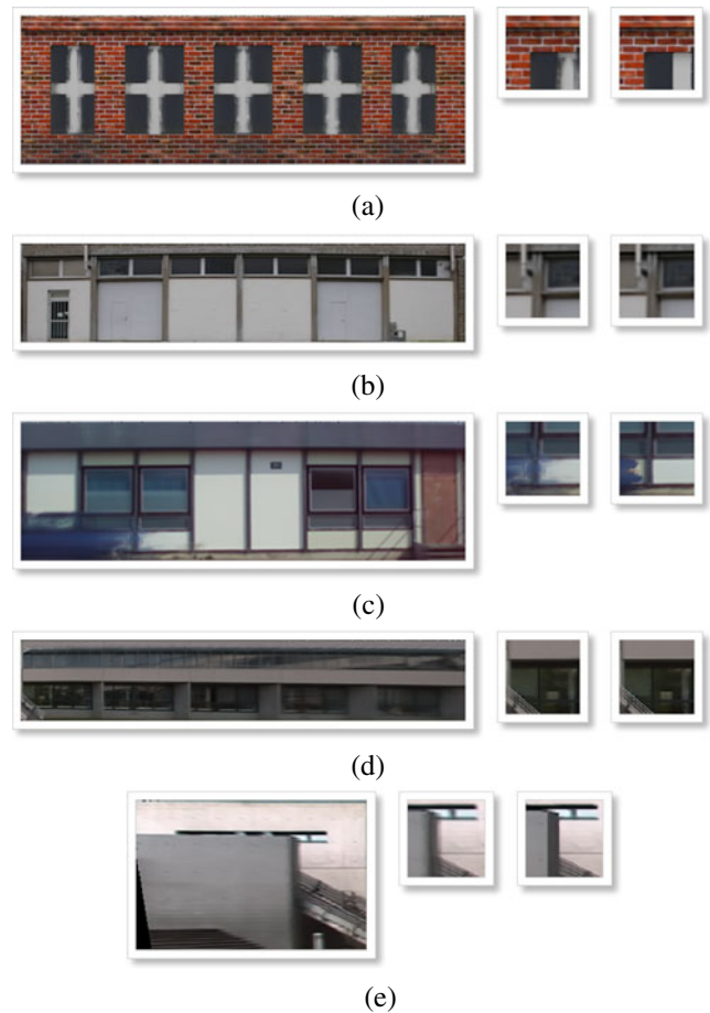
Fig. 14 Texture fusion—algorithm by Teller et al.. The left column presents the textures computed using Teller's algorithm. The central column represents a small detail from each of these textures, and the right column the same detail computed with our algorithm (best viewed in the electronic version of the paper)
