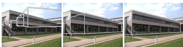
Fig. 4 Automatic initial registration: example of failed pose computation with arbitrary keyframe selection ( left ), false proposition (too many RANSAC iterations, center ) and obtained registration validated by the user (small number of RANSAC iterations, right )
