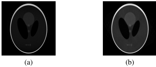
Figure 2. Images reconstructed with the BFP (a) and the SART (b) algorithms using the sinogram 1(b).
