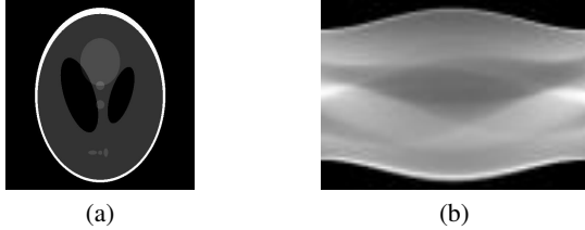
Figure 1. (a) Original domain. (b) Acquisition of the original domain following 90 angles (X-axis) of 64 samples (Y-axis).
