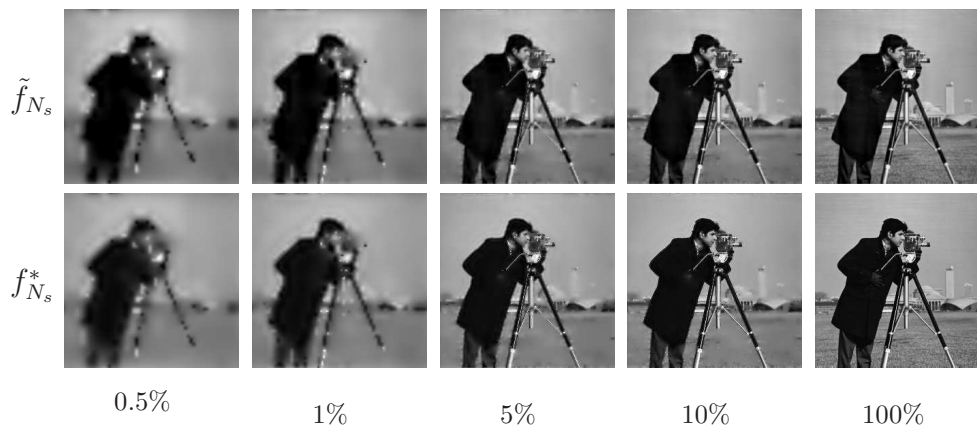
Figure 7: Reconstruction of the cameraman image f using different percentages of the highest c_{kij} . Upper line shows the straightforward progressive synthesis \tilde{f}_{N_s} . Bottom line shows the corrected reconstruction f^*_{N_s} using the dual frame. PSNR for the upper/lower image is from left to right: (19.2 dB/19.5 dB), (20.4 dB/20.8 dB), (24.08 dB/25 dB), (25.8 dB /27.5 dB), and (27.9 dB/296 dB).
