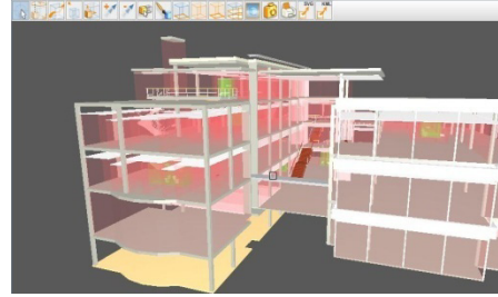
Fig. 5. Structural view of a building. This view is required for structure engineers. The corresponding graph provides all elements needed to make structure calculations.
