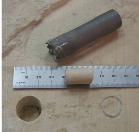
Figure 7: Coring Bit and Resulting Hole and Core
