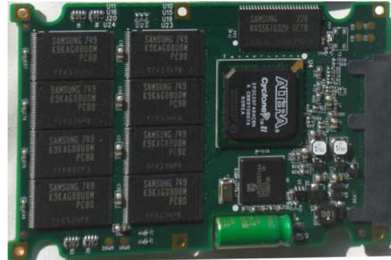
Figure 1: Internal view of the Memoright 32 GB SSD
