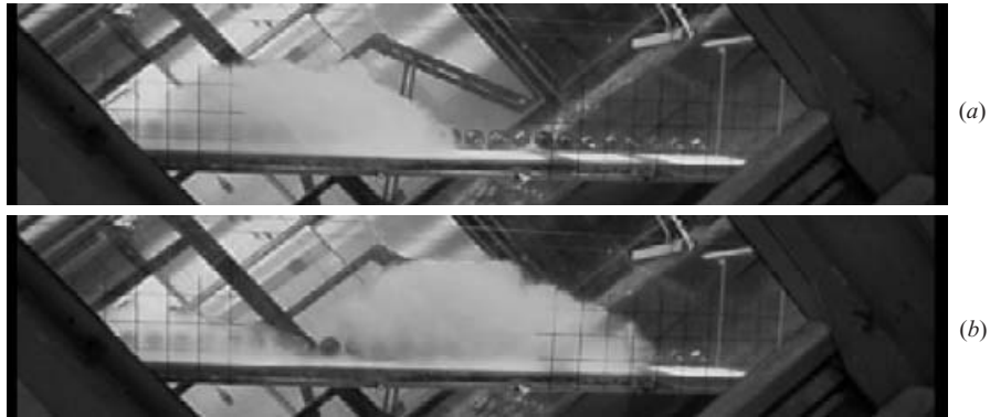
FIGURE 6. Side view of a saline cloud moving down a smooth slope of angle 32^\circ : (a) the front is 120 cm from the gate, (b) the front is 155 cm from the gate. The grid lines on the image are a 5 cm mesh.
