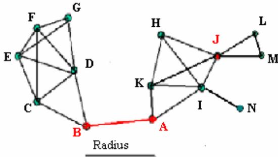
Figure 1. Unit graph representation of multi-hop wireless network
