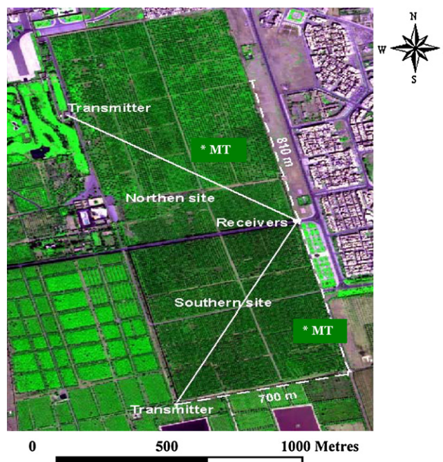
Fig. 1. Overview of the location site and the experimental setup (Quickbird image). The locations of LAS and micrometeorological towers (MT) are marked.
