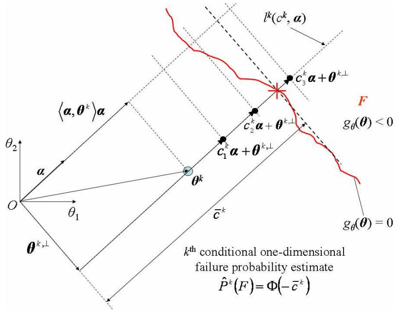
**Fig. 1.1'.** The Line Sampling procedure (Pradlwarter et al. 2005)
