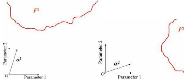
**Fig. 1.3.** Examples of possible important unit vectors  $\alpha^1$  (left) and  $\alpha^2$  (right) pointing towards the corresponding failure domains  $F^1$  (left) and  $F^2$  (right) in a two-dimensional uncertain parameter space
