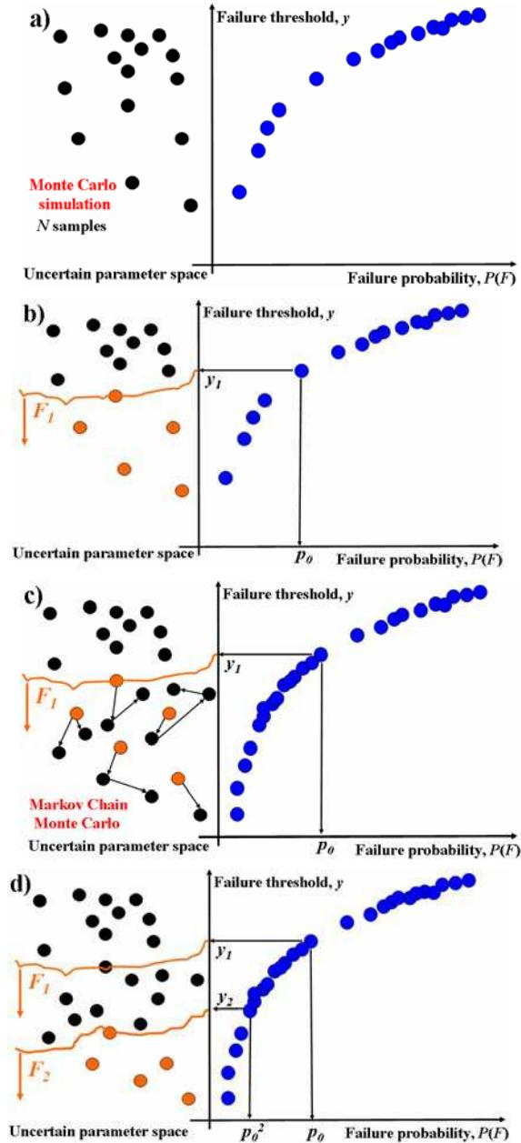
**Fig. 1.2.** Illustration of the SS procedure: a) Conditional level 0: Standard Monte Carlo simulation; b) Conditional level 0: adaptive selection of  $y_1$ ; c) Conditional level 1: Markov Chain Monte Carlo simulation; d) Conditional level 1: adaptive selection of  $y_2$  (Au 2005)
