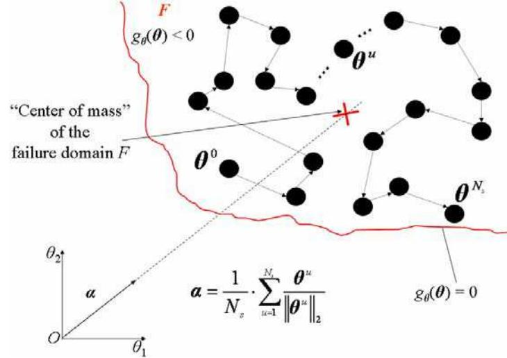
**Fig. 1.4.** Line Sampling important unit vector  $\alpha$  taken as the normalized “center of mass” of the failure domain  $F$  in the standard normal space. The “center of mass” of  $F$  is computed as an average of  $N_s$  failure points generated by means of a Markov chain starting from an initial failure point  $\theta^0$  (Koutsourelakis et al. 2004)
