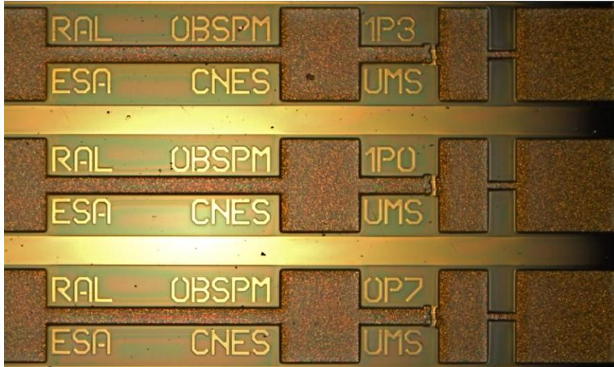
Figure 2.66: Photo of the mixer chips with three different anode sizes on a tile of the UMS fabricated wafer.
