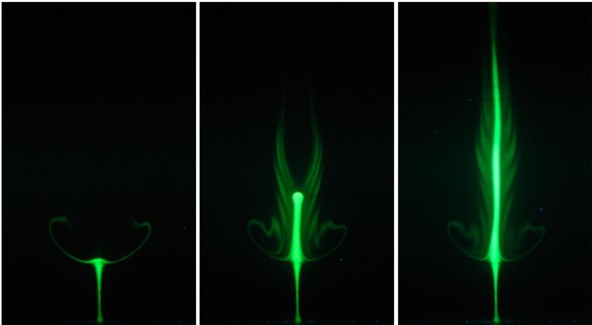
Figure 1: Temporal evolution of a light dye injected below the vortex breakdown and which pierces through the bubble without its destruction. Density difference:  $\Delta\rho/\rho_0 = -2.3 \cdot 10^{-4}$ .  $Re = 2423$ .
