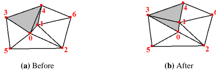
Fig. 4 Flip operation resulting from crossing the base line of the triangle during node 0 's movement towards node 2
