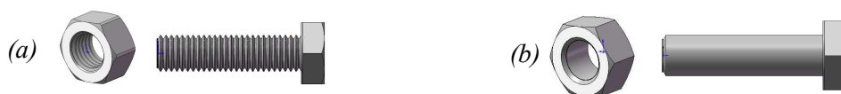
Figure 7. Two representations of a screw and a nut (a) detailed model, (b) idealized model.
