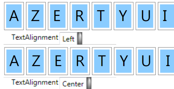
Figure 7. The text alignment is set to left for each letter instead of centered. The difference is not really perceptible for larger letters but noticeable on the 'I' key.
