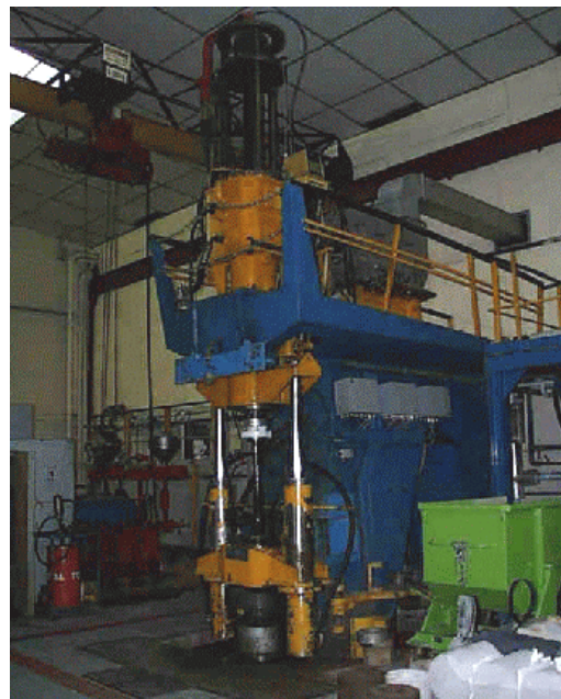
Figure 17 : Full Scale Drilling Test stand
