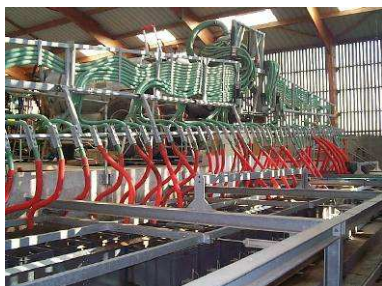
Photo 2: Detail of test bench for trailing hoses spreader
