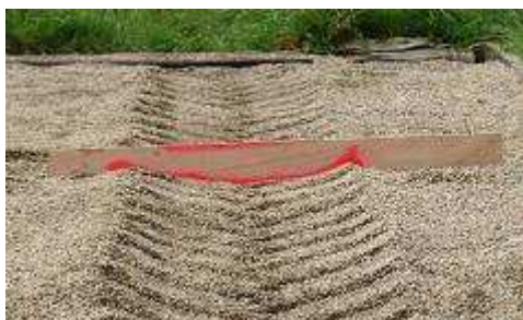
Photo 7: Tracing of rut profile
