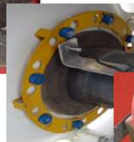
(c) – inductive sensor for spreader speed measure
