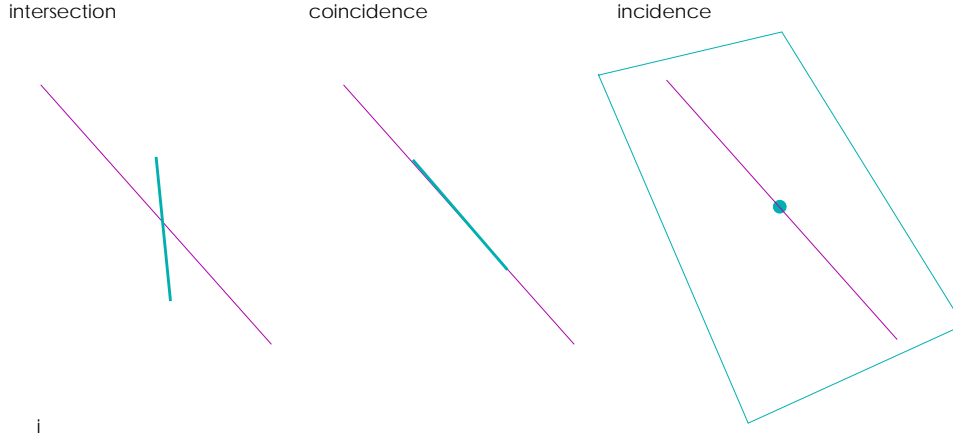
Figure 2.15: Intersection, incidence, and coincidence relation between linear geometric features, i.e. points, lines, planes, . . .
