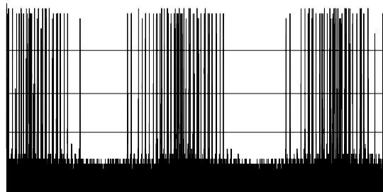
Figure 8. Chaotic signal in the case where D = 0.0535 . Abscissa: 5 \mu\text{s} per division; ordinate: 2 V per division.
