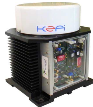
Figure 2. General view of the K2Pi radar.
