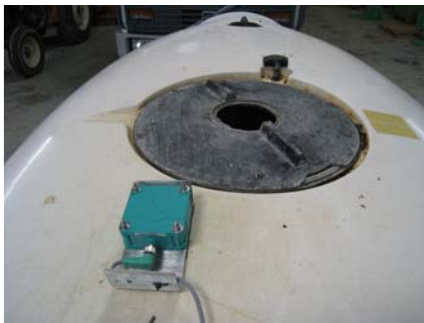
Figure 4: Tank level sensor © Cemagref 2009
