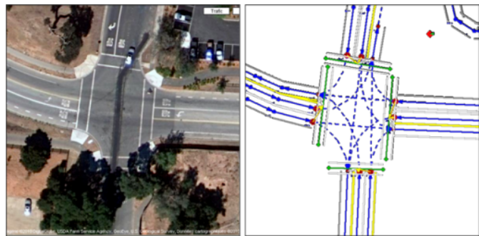
Figure 1. This intersection (satellite imagery on the left, RNDF representation on the right) has 4 roads, 8 entrance lanes, 4 exit lanes and 12 crossing connections. The blue arrows represent the centre of lanes and the dotted arrows inside the intersection area are the exemplar paths generated for each crossing connection. The green lines show the position of crosswalks. The red dots are the delimiters between the inside and the outside of the intersection.
