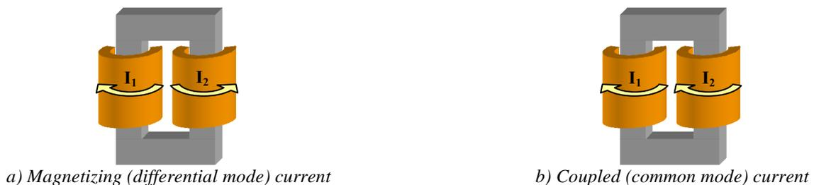
Figure III.4: Current directions when simulating coupled and magnetizing currents.
