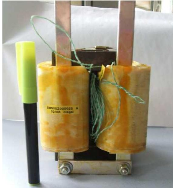
Figure III.12: InterCell transformer.
