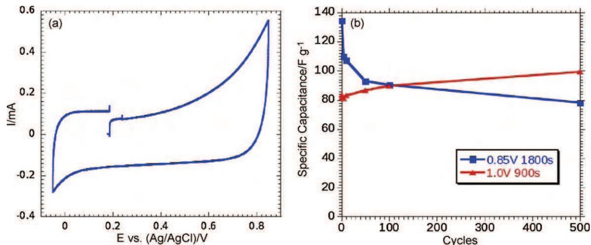
**Fig. 4.** CV of  $\text{MnO}_2$ -coated Ni nanorods (single-step method, 1 V for 900 s) in  $\text{K}_2\text{SO}_4$  0.1 M (a). Evolution of capacitance upon cycling of an  $\text{MnO}_2$ -coated Ni nanorods electrode (b). Deposition performed by single-step potentiostatic method at 1.0 V for 900 s (triangles,  $m_{\text{MnO}_2} = 0.0177$  mg) and at 0.85 V for 1800 s (squares,  $m_{\text{MnO}_2} = 0.0545$  mg).
