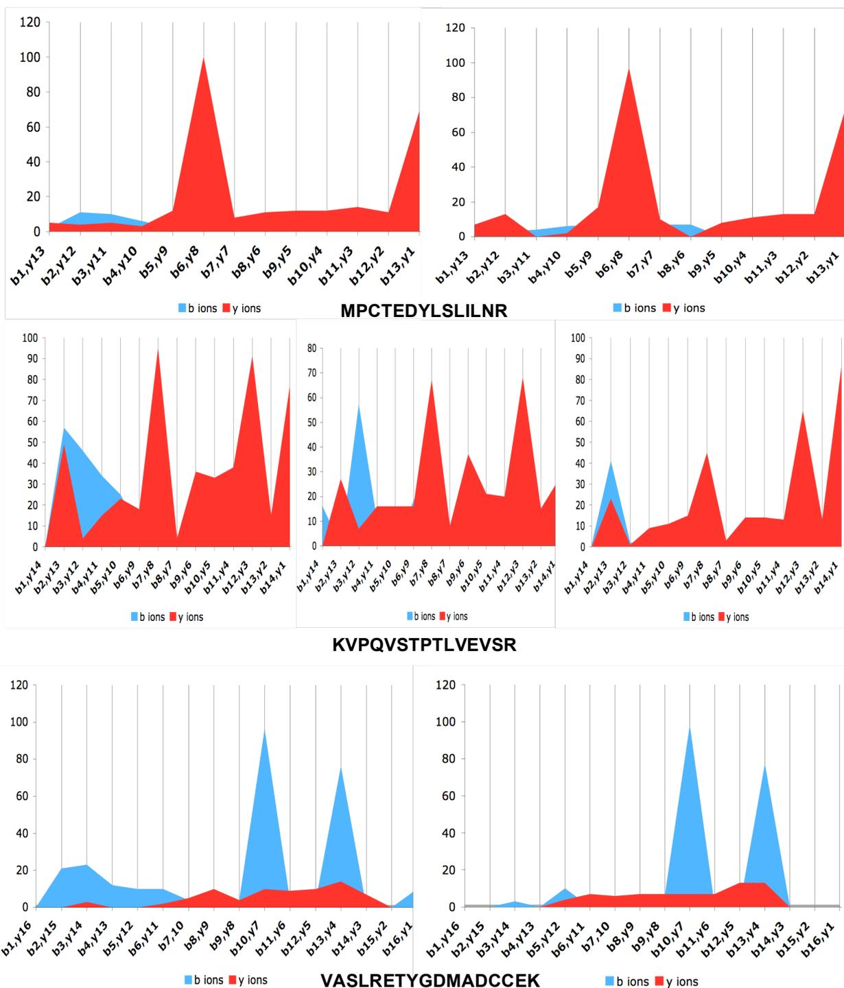
**Fig.4.5** graphic representation of ion intensities in function of the different  $b_n$  and  $y_n$  fragments. The resulting red curve is related to the  $y$ -type ions and the blue curve is related to the  $b$ -type ions
