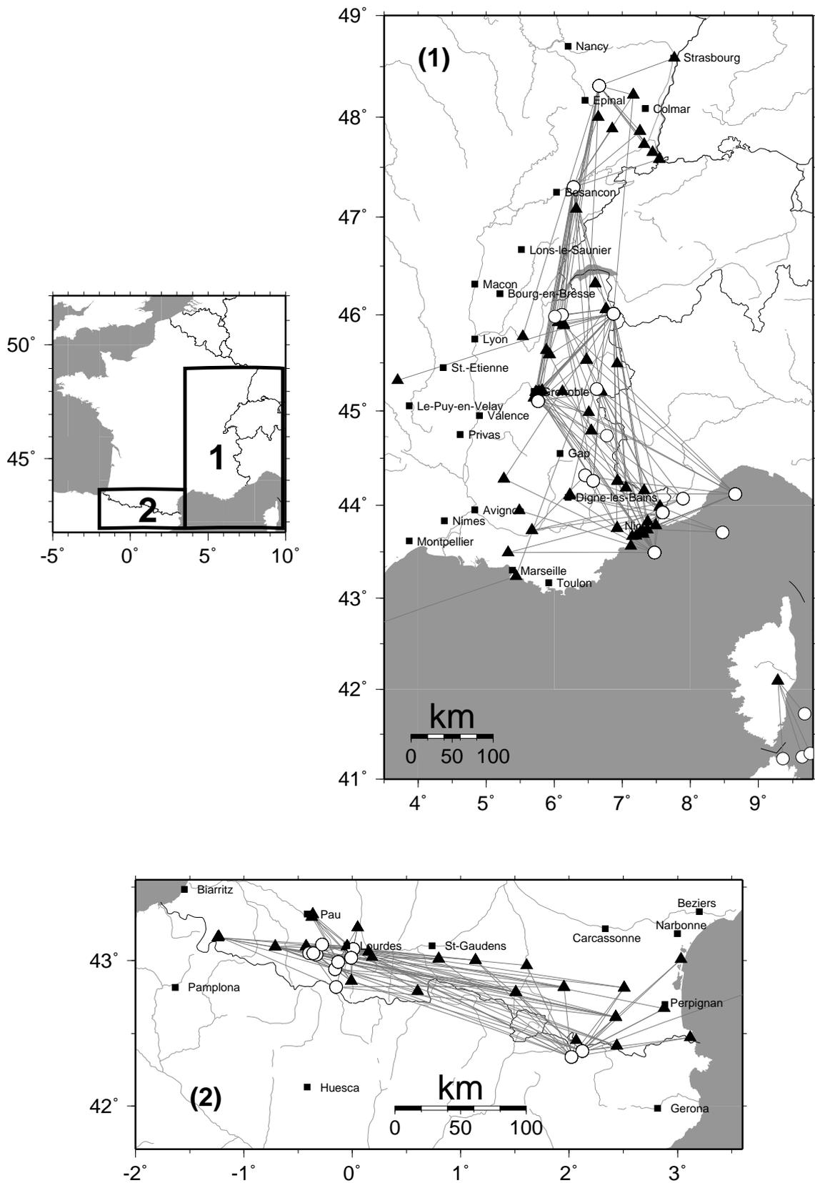
Figure 1: Epicentral (circles) and station (triangles) locations and travel paths (lines) of the records used for this study.
