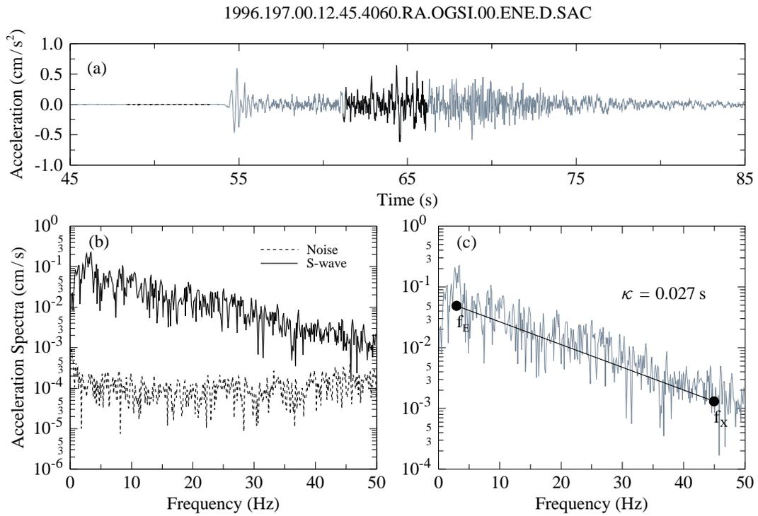
Figure 2: Example of direct shear-wave and noise spectra computed from a record that shows a clear high-frequency linear trend. Also shown are the intervals used to estimate the pre-event noise and the direct shear-wave spectra (black parts of acceleration time-history) and the frequencies  $f_E$  and  $f_X$  chosen by one of the analysts (the other analysts chose similar  $f_E$  and  $f_X$  for records such as this).
