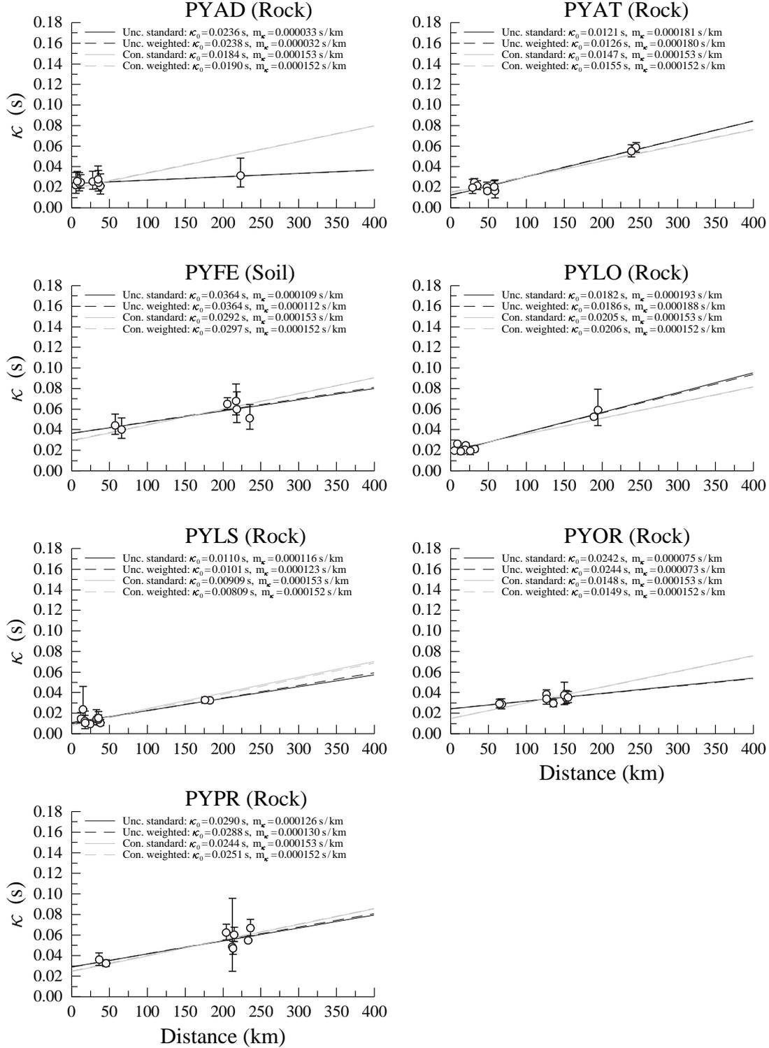
Figure 8:  $\kappa$  estimates and their  $\pm 1$  standard deviations for stations located in the Pyrenees. Also shown are the fitted linear relations. Four best-fit lines were fitted for each station: two (using standard and weighted regression) in which  $m_\kappa$  was allowed to vary (black) and two (using standard and weighted regression) in which  $m_\kappa$  was constrained to the value from the regional analysis shown in Figure 6 (grey).
