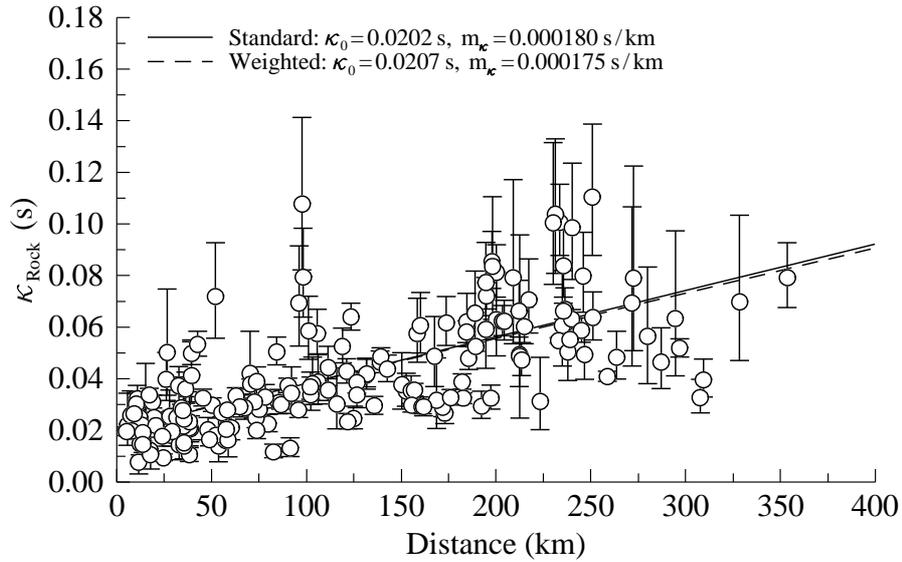
Figure 5: Distance dependence of  $\kappa$  for all stations for soil and rock conditions. The vertical lines represent the standard deviation of six independent measurements of  $\kappa$  (three estimates, two horizontal components). Results for  $\kappa_0$  and  $m_\kappa$  from standard (solid line) and weighted (dashed line) least squares regressions are shown in the legend of each plot.
