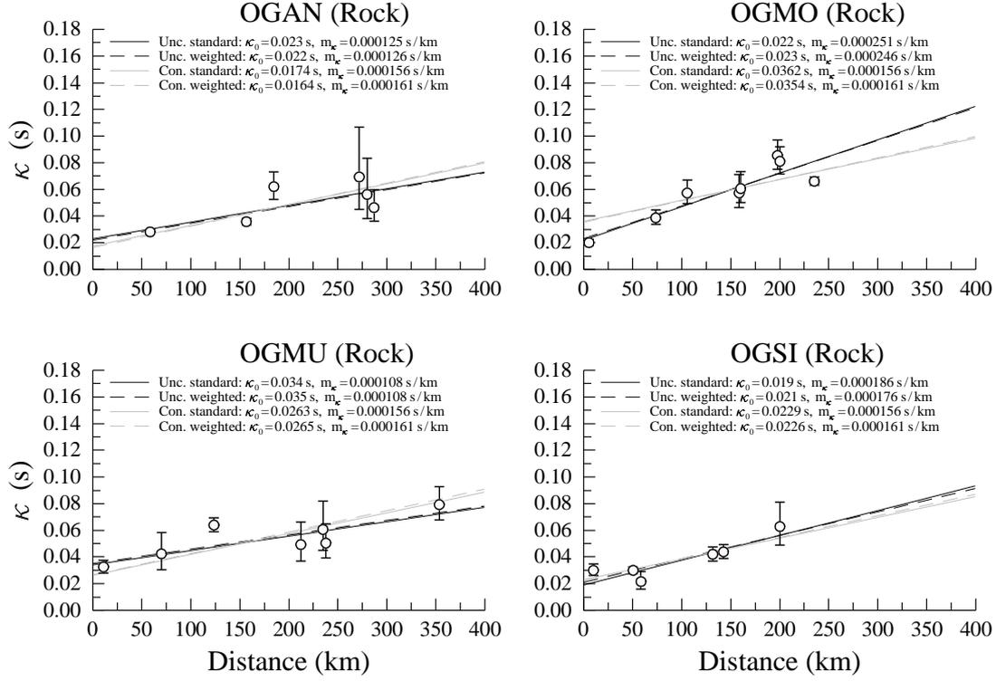
Figure 7:  $\kappa$  estimates and their  $\pm 1$  standard deviations for stations located in the Alps. Also shown are the fitted linear relations. Four best-fit lines were fitted for each station: two (using standard and weighted regression) in which  $m_\kappa$  was allowed to vary (black) and two (using standard and weighted regression) in which  $m_\kappa$  was constrained to the value from the regional analysis shown in Figure 6 (grey).
