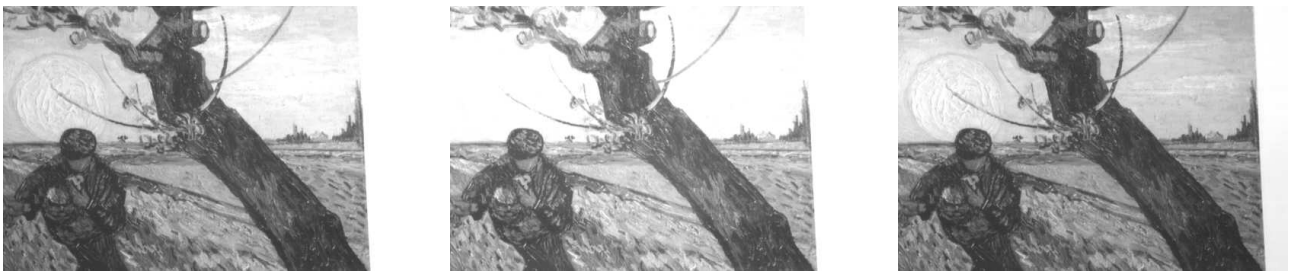
Figure 16: Complex illumination variation. The reference image is on the left (image # 0), the light source is furthest right for this image. For the image in the middle the light source is in front of the scene (image # 6). For the one on the right the light source is furthest left (image # 11).
