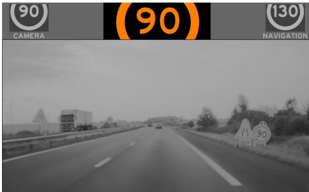
Fig. 8. Conflicting situation successfully managed with fusion. Camera-based system detected the road sign on the image and recognized a speed limit of 90 km/h due to roadwork. On the contrary, navigation locating the vehicle on a highway output a limitation of 130 km/h. After combining the two sources of information, the decision unit chose the most likely value, which was 90 km/h.
