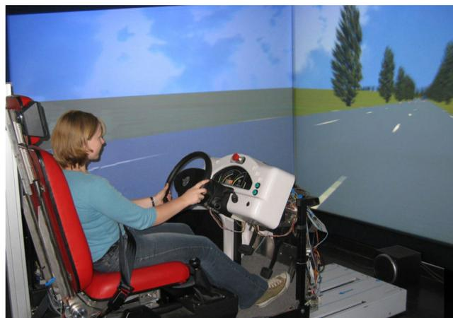
Fig. 4.1: Fixed-base mini-driving simulator.(c) 2007 MSIS INRETS
