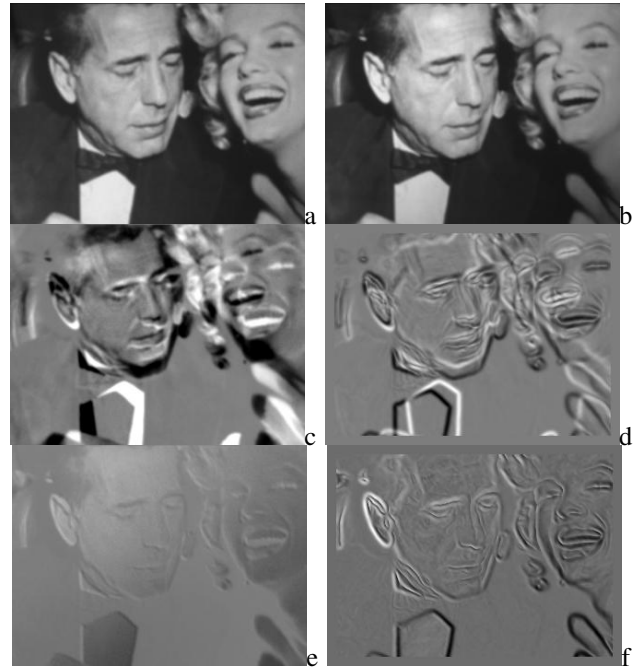
Fig. 10. Influence of luminance variation (a) desired image (b) final image \mathbf{r}^* (c) initial error in the intensity space (\mathbf{I}(\mathbf{r}) - \mathbf{I}(\mathbf{s}(\mathbf{r}))) and (e) initial error on the norm of the gradient used in the control law (\|\nabla \mathbf{I}(\mathbf{r})\|^2 - \|\nabla \mathbf{I}(\mathbf{r}^*)\|^2) (d) final error in the intensity space and (f) final error on the norm of the gradient used in the control law.
