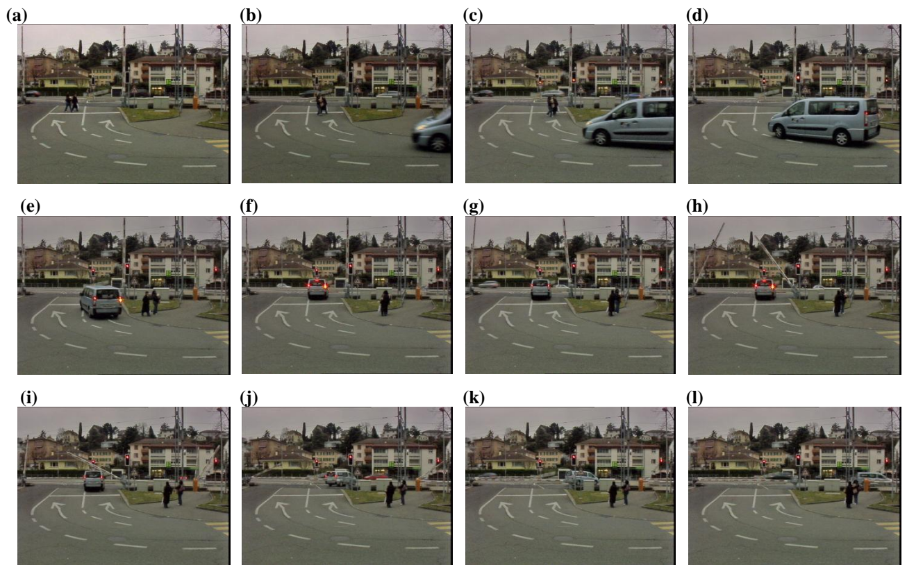
Figure 5. An example of hazardous situation scenario detected from cameras devices. (a) Pedestrians near a crossing, (b) appearance of a car, (c) A car approaching the crossing (first level of red-light sensor), (d) A car approaching the crossing (second level of red-light sensor), (e) A car on the crossing (third level of red-light sensor: a mandatory stop), violation of red-light, (f) A car stopped on the critical area, (g) Start of lowering barriers, (h) Car driver is still on the dangerous zone, (i) A barrier is lowered and jammed on the car, (j) Car driver has forced the barrier: It is full track, (k) The car passing the hazardous area, (l) A free and safe level crossing (barriers are still lowered).
