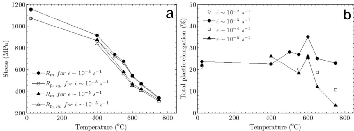
**Fig. 2:** Evolution of (a) the ultimate tensile strength ( $R_m$ ) and yield strength ( $R_{p0.2\%}$ ) and (b) of the total plastic elongation according to the temperature and for various strain rates. J05 steel.
