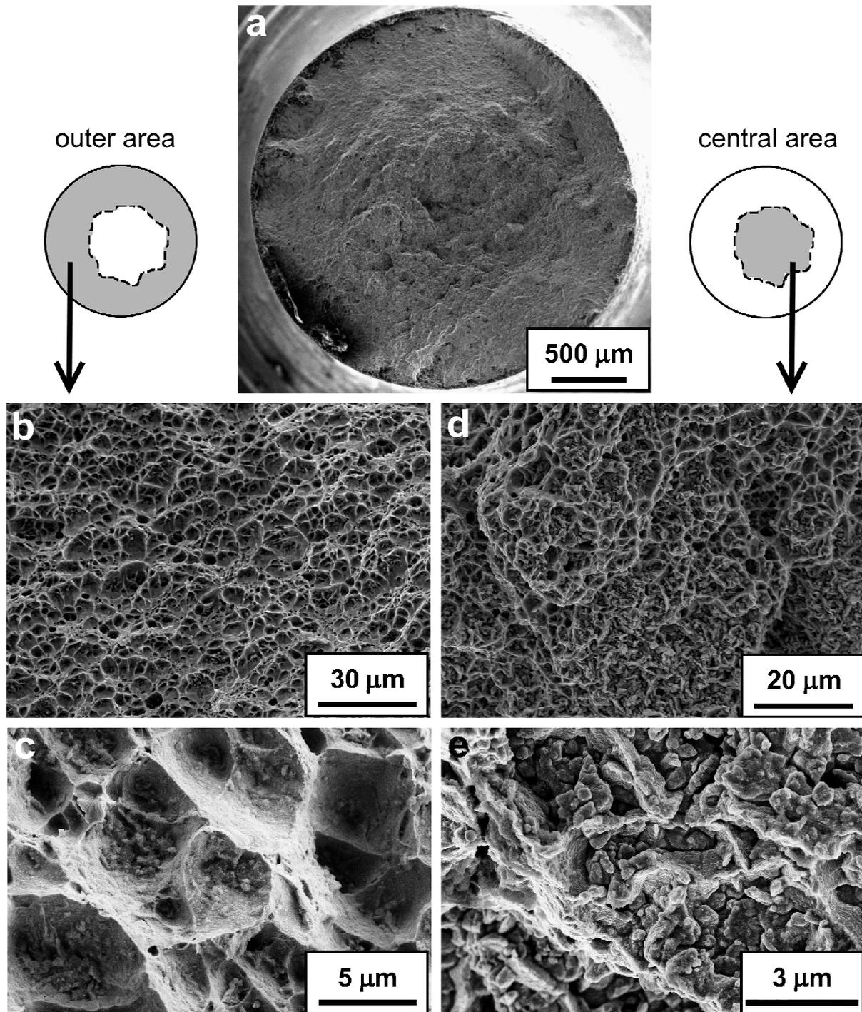
**Fig. 5:** SEM images of the fracture surface of a J05 specimen tested in tension at 650°C and  $10^{-5} \text{ s}^{-1}$ . Overall view (a) and zooms in the outer area (b,c) and in the central area (d,e). The two schemes describes respectively the outer are where dimples are predominant (left) and the central area where intergranular decohesion is observed (right).
