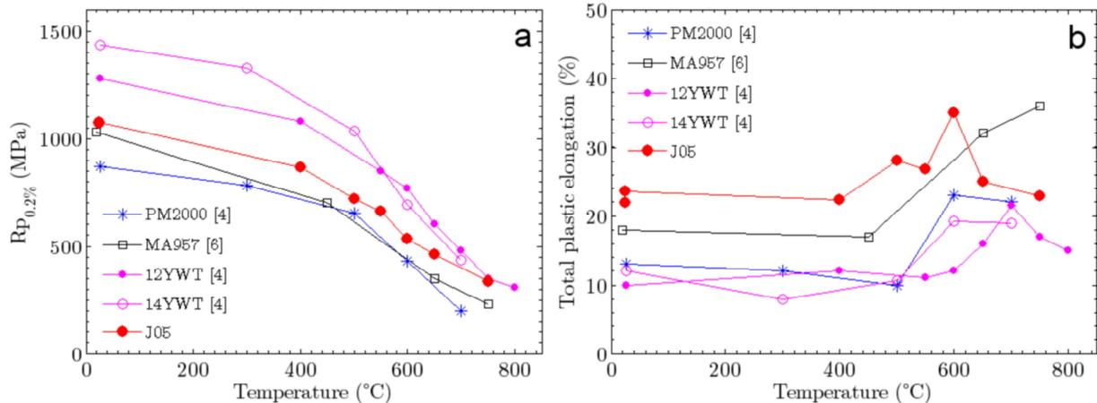
**Fig. 3:** Evolution of (a) the ultimate tensile strength ( $R_m$ ) and yield strength ( $R_{p0.2\%}$ ) and (b) of the total plastic elongation according to the temperature and for various strain rates. Various ferritic ODS steels of literature.
