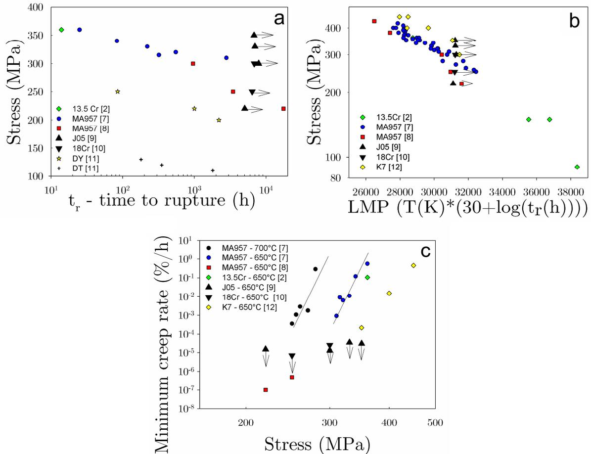
**Fig. 4:** Creep results for different ferritic ODS steels. Lifetime diagram at 650°C (a), Larson-Miller diagram for temperatures between 600°C and 900°C (b) and minimum creep rate diagram at 650°C (and 700°C) (c).
